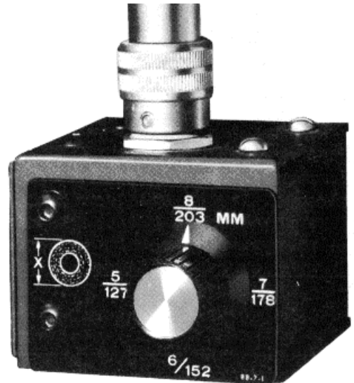
Fig. 25D. Safety interlock at rear wheel guard prevents overspeeding of grinding wheels.
